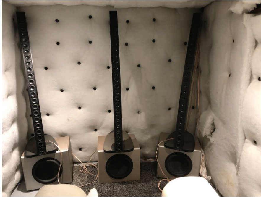
Figure 2: Speaker set up in hemi-anechoic room
