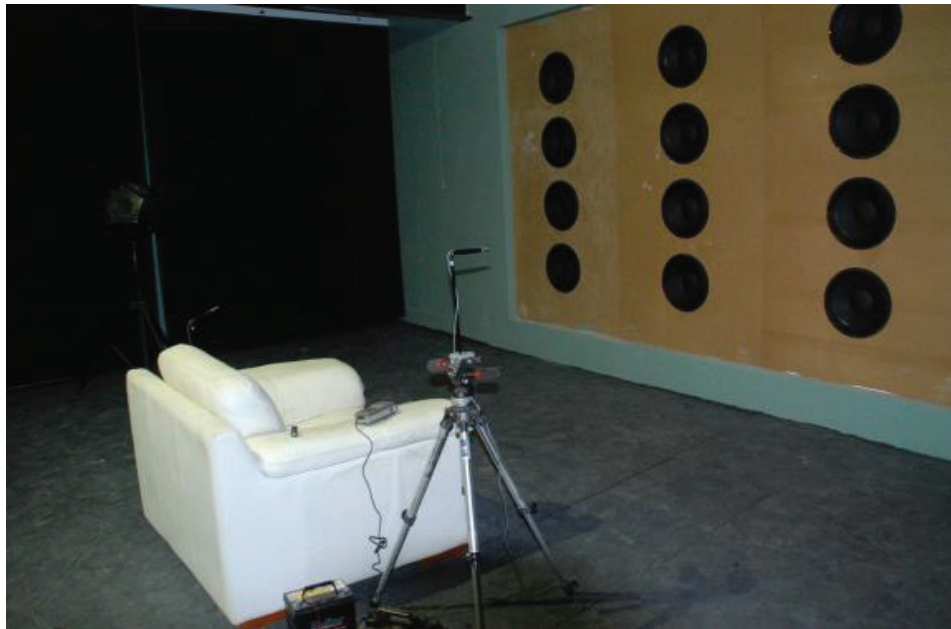
Figure 1: Test set up in Reverberation Room
